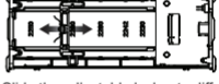
Slide the adjustable locker to different lockpoints (2230 / 2242 / 2260 / 2280 / 22110) according to your SSD's length.
